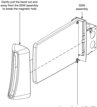
Unscrew the two 4-40 x 1/2" screws to remove the acrylic.
