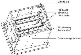
**NOTE:** Ensure that the unit is properly grounded by connecting the chassis ground lug to an earth ground (building steel).
