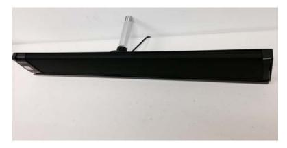
**Step 1:** Screw the (2<sup>nd</sup>) mounting flange into the ceiling (\*please make sure to use the appropriate screws for the ceiling materials and make sure to allow sufficient space behind the rear of the mic to be able to insert the rear panel screws -approx 2" or more).
