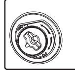
2. Select the tap position by removing the rubber plug on grille to access rotary switch. Switch is preset to maximum tap setting in 70.7 V mode. Select desired setting and reinsert rubber plug. **Note:** The grille-mounted tap switch cover is keyed; be sure flat edge of plug lines up with flat edge of hole in grille.
