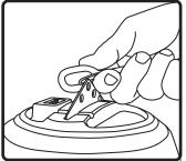
**10.** Attach the safety cable to one of the secondary holes in the hanging bracket.
