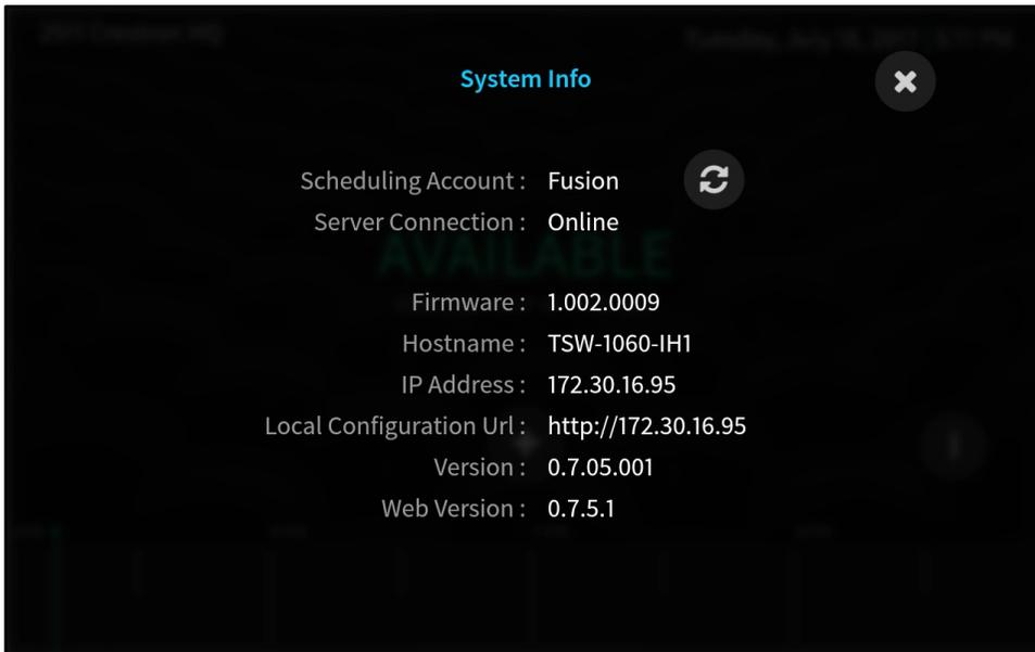
The **System Info** screen displays the scheduling calendar source and the server connection status. Tap the refresh button
