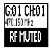
Use this to turn on a transmitter without interfering with the RF spectrum.
