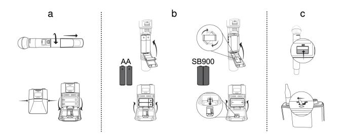
The transmitter runs on two AA batteries or the Shure SB900 rechargeable battery. Use the included AA battery adapter when using batteries other than the Shure SB900.
