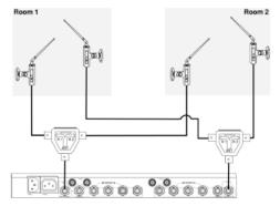
When using powered antennas, use UA221-C-J or UA221Z-C-J.
