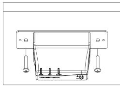
4. Attach the desired decorator style faceplate (not supplied). GLS-PART-CN Installed on Surface with Faceplate
