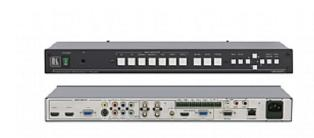
The VP-437xI is a 7-input scaler/switcher for composite video, s-Video (Y/C), component video, computer graphics video and HDMI with unbalanced stereo and S/PDIF audio signals. It scales the selected video signal to a computer graphics or HDTV output resolution, embeds the audio and outputs an HDMI signal. The VP-437xI is the same as the VP-436 with the addition of Ethernet control
