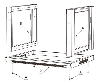
1: Insert the Left Frame (#5) and the Right Frame (#6) into the Bottom Panel (#2), Secure with M5 Screws (A) .
