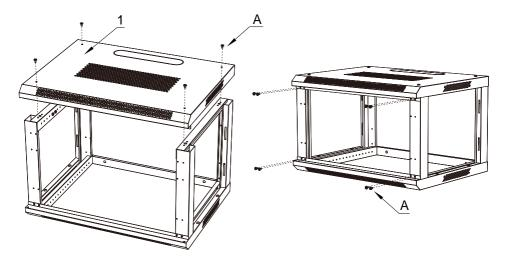
2: Place the Top Panel (#1) onto the Left Frame (#5) and the Right Frame (#6). Secure with M5 Screws(A).
