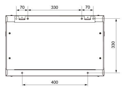
1: Attach the rack to a wall or other suitable mounting surface using M10 Expansion screws(G). The mounting hole distance is shown in Fig, apart to accommodate standard stud placement as reflected in the diagram.
