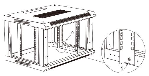
3: Install the 4 Vertical Mounting Rails (#9) into place at the desired depth using M5 Screws(A)for each Vertical Mounting Rails (#9). **Note:** Please consider the equipment you plan to install within the enclosure while deciding the appropriate mounting depth. Make sure the rail depth on both sides of the cabinet is the same.
