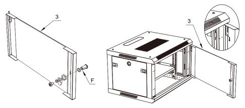
7: Install the Front Door Lock (F) on the Front Door (#3).
