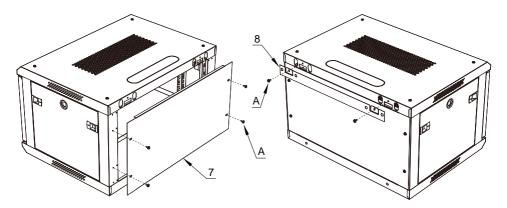
9: Install the Rear panel ( #7) and the Rear suspension (#8) ,Secure with M5 Screws(A) .
