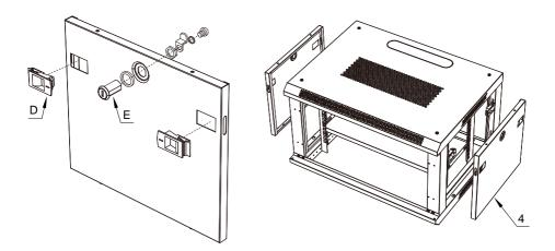
5: Install the Side Panel Latches (D) and the Side Panel Lock Kit (E) on the two Side Panels (#4).
