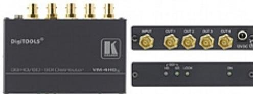
The **VM-4HDxI** is a high-performance distribution amplifier for 3G HD-SDI signals. The unit takes one input, provides reclocking and equalization and distributes the signal to four identical outputs.
