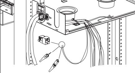
Terminate the fibers with an appropriate connector. Mount each connector in the panel.
