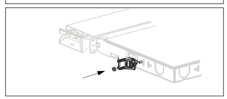
Place the strain relief bracket near area where the cable will enter the enclosure. Fasten with #10-32 hex nut.
