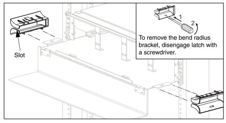
To install the bend radius brackets, slide the bracket onto tab with the slot facing outside then snap in place. (FMD SERIES ONLY)
