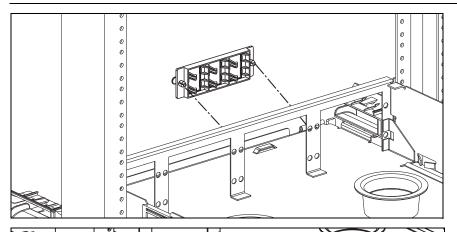
Insert the panels into the enclosure as shown. Once mounted, push the latches in to secure the panel.
