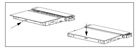
To engage the cover, slide forward until the cover slides under the front tabs then secure in place with #10-32 screw.
