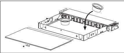
Determine where the spools will be located. Remove the liner from the tape on each spool and place them inside the enclosure.
