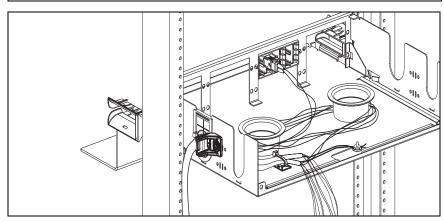
Gently loop the excess fiber around the spools. Replace the cover after all fibers are looped around the spools
