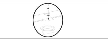
Install the hex nut and washer. This will be used to secure the strength member that comes out of the cable.
