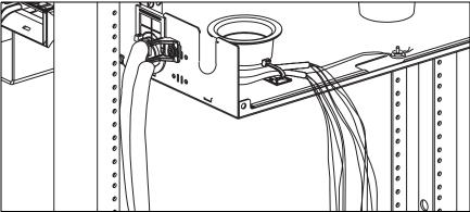
Insert cable through the grommet. Secure the cable to the strain relief bracket using a cable tie. Strip 1 meter of jacket from the end of the cable. Attach the strength member of the cable to the #10-32 stud and #10-32 hex nut. Use the adhesive mount and cable tie to secure the cable between the#10-32 stud and the grommet.
