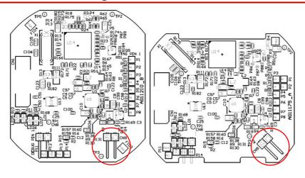
Jumper link **CN9** on the main PCB board lets you reset the network settings to factory default. To reset, short the link for 10s whilst applying power to the unit.
