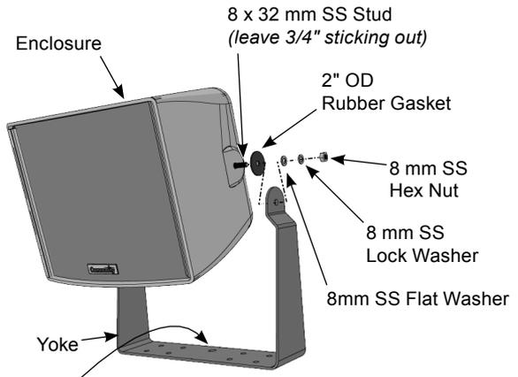
Mount yoke to the surface using holes aligned with large center hole as primary mounting points - these are aligned with the center of gravity. Use other holes as secondary reinforcement. Orient angled side to the front of the loudspeaker if the yoke is mounted below the enclosure.
