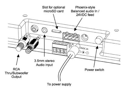
The Phoenix-style connector allows direct wire connections for balanced audio input, and DC power (24V). The ground pin is shared between audio and power input.
