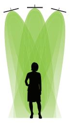
Many variations of these basic designs are possible — this manual is intended to act as a guide. In considering different ways to install the Audio Spotlight speakers, keep the lighting analogy in mind. More often than not, Audio Spotlight should be thought of in lighting design terms, not in loudspeaker terms.
