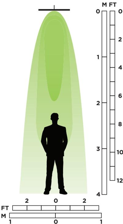
The loudest sound area is directly in front of the speaker panel at a distance of 1-2m. Sound levels outside the beam are reduced by over 90%.
