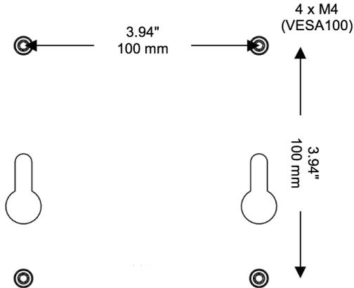
**NOTE:** When using the keyhole mounts for overhead mounting, a secondary fastener, bumper, or retainer **MUST** be used in case the speaker is inadvertently moved, to prevent falling.
