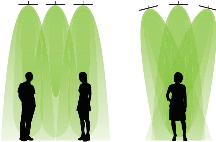
Many variations of these basic designs are possible — this manual is intended to act as a guide. In considering different ways to install the Audio Spotlight speakers, keep the lighting analogy in mind. More often than not, Audio Spotlight should be thought of in lighting design terms, not in loudspeaker terms.
