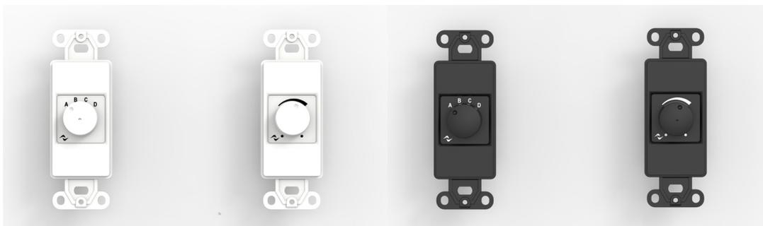
The WMP controllers are a series of wall-mounted solutions aimed at remotely controlling system functionalities, such as zone level control and source selection. These passive controls are sharable over the network, meaning that a passive wall controller can be connected to one amplifier via GPI and control the parameters of other devices in the same network.
