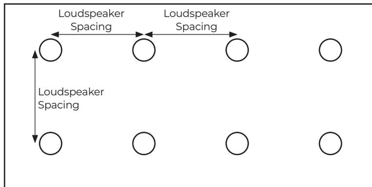
D. After the last loudspeaker is placed, center the loudspeakers in that row to create new offset distances out from each wall, which may be unique from 1/2 LSD.
