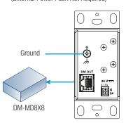
Connection to DigitalMedia Receiver (External Power Pack Required)
