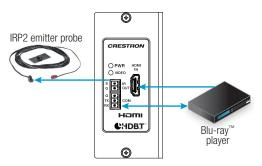
1. The IR OUT port and the COM (RS-232) port are enabled only when the DM-TX-4K-100-C-1G connects to an Ethernet-enabled DigitalMedia receiver or switcher that is addressable from a Crestron control system.
