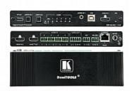
DSP-62-AEC is a member of the Kramer XSPerience family of DSP products. DSP-62-AEC is an advanced, professional 6 x 2 audio matrix switcher that includes multi-channel DSP, AEC (Acoustic Echo Cancellation), HDMI de-embedding, and class compliant USB audio interface. The comprehensive and user-friendly graphic interface makes configuring every detail of your audio system intuitive and easy
