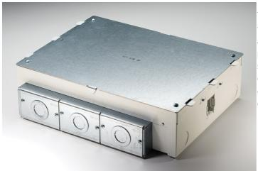
The Evolution™ Series Six Gang Floor Box has been designed to be installed in concrete, raised, and wood floor applications. The box has a fully finished interior to assist plugging and unplugging of devices. Designed to work with standard size wall plates. It comes complete with all components needed for initial installation. The floor box is compatible with Walkerflex Modular Wiring System. Custom options are available upon request.
