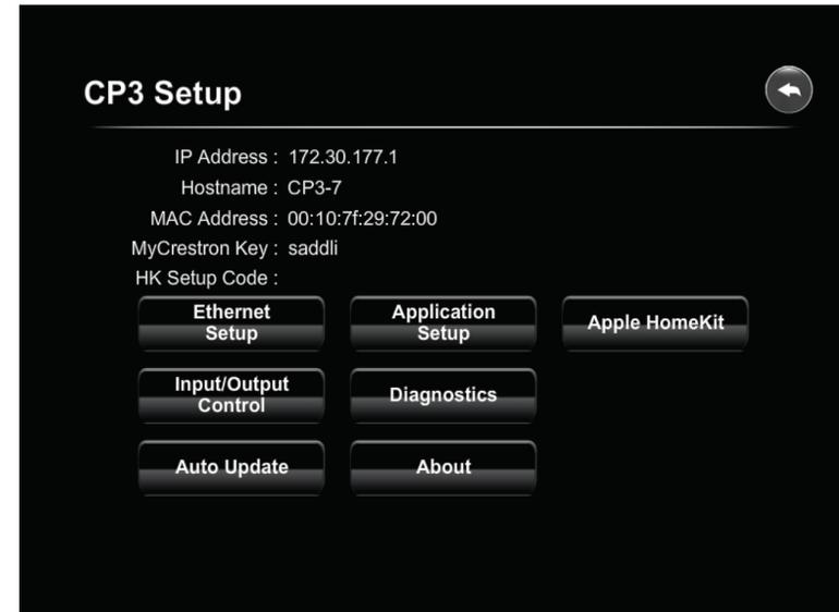
The Setup page displays the IP address, hostname, and MAC address of the control system, as well as a key that is used to register the control system with the MyCrestron service.
