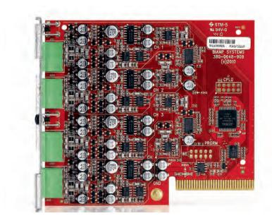
The Tesira® SIC-4 is a modular analog input card for use with Tesira SERVER and SERVER-IO devices. Each SIC-4 provides 4 channels of Mic or Line level audio input. The inputs are electrically balanced and provided on plug-in barrier strip connectors. Software control of each input includes gain with clip indicator, +48V phantom power, mute, level and signal invert.
