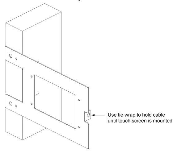
For post-construction applications, use the TSW-UMB-PMK as a cutout template by turning it to face the wall, ensuring it is level and temporarily tacking it to the wall with finishing nails (not included) in the smaller holes around the cutout opening.
