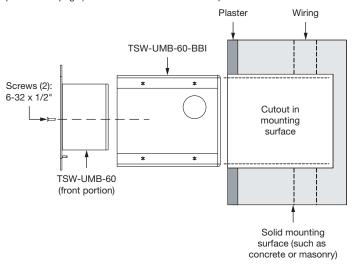
**NOTE:** The TSW-UMB-60-BBI can also be mounted vertically for use with the TSW-560P portrait touch screen. For this installation, ensure that the "TOP" text on the front of the TSW-UMB-60 and the "TOP" text on the inside of the TSW-UMB-60-BBI are facing to the right, and then install the TSW-UMB-60-BBI into an appropriately sized cutout in the mounting surface. (Rotate the product 90° to the right to determine the necessary cutout dimensions for portrait mounting.)
