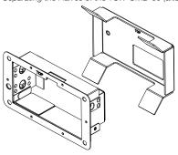
**NOTE:** The rear portion of the mounting bracket can be saved for possible future use. Only the front portion is required for installing the TSW-UMB-60-BBI.
