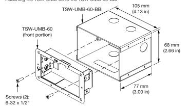
**NOTE:** Remove the appropriate knockouts on the TSW-UMB-60-BBI before installation.
