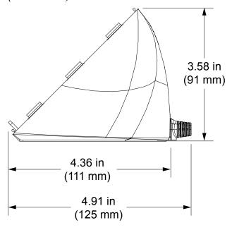
TSW-730-TTK Overall Dimensions (Side View, Shown with Rear Wire Grommet, Swivel Mount and Touch Screen Installed)
