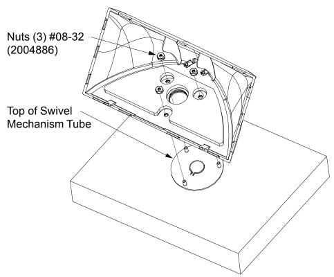
2. If cables are routed to exit through the bottom of the TSW-730-TTK, feed the full length of the cable through the swivel mechanism tube.
