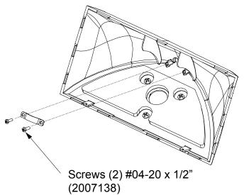
The illustration above shows metal wire capture installed "bow" side up. When fewer cables are routed through the rear of the TSW-730-TTK, installing the metal wire capture "bow" side down holds the cables more securely.
