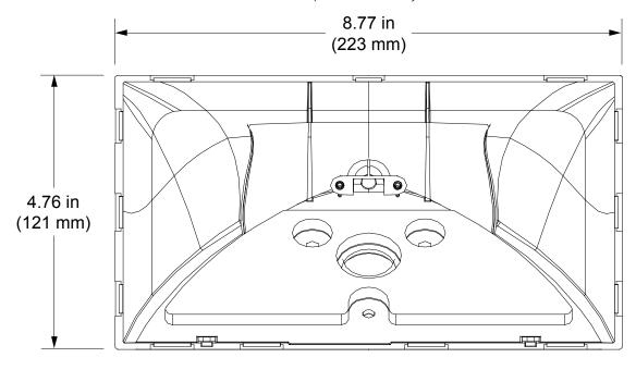
TSW-730-TTK Overall Dimensions (Side View, Shown with Rear Wire Grommet)
