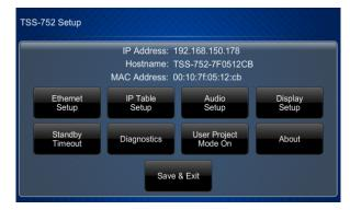
To access the setup screens after the TSS-752 boots to the Crestron Fusion® Cloud software "Offline" screen, press the hard keys labeled below as 1, 2, 3, and 4 in sequence, twice (press 1, 2, 3, 4, 1, 2, 3, 4) within a 5-second period.
