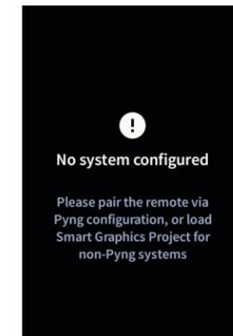
The TSR-310 may be set up to run the built-in Performance UI software for controlling a Crestron Home OS system or set up to run a custom Smart Graphics® technology project.
