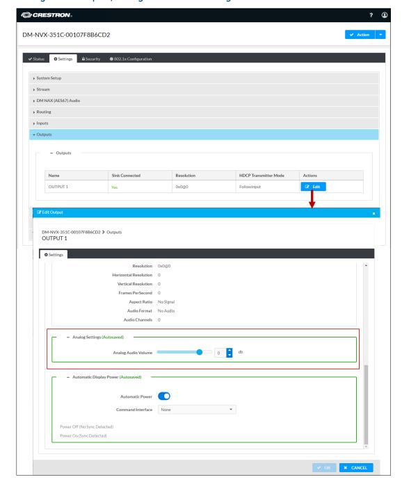
Settings Tab – Outputs, Analog Audio Volume Configuration
