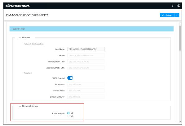
**NOTE:** When a different IGMP snooping support version is selected, the DM NVX device must be rebooted in order for the change to take effect.
