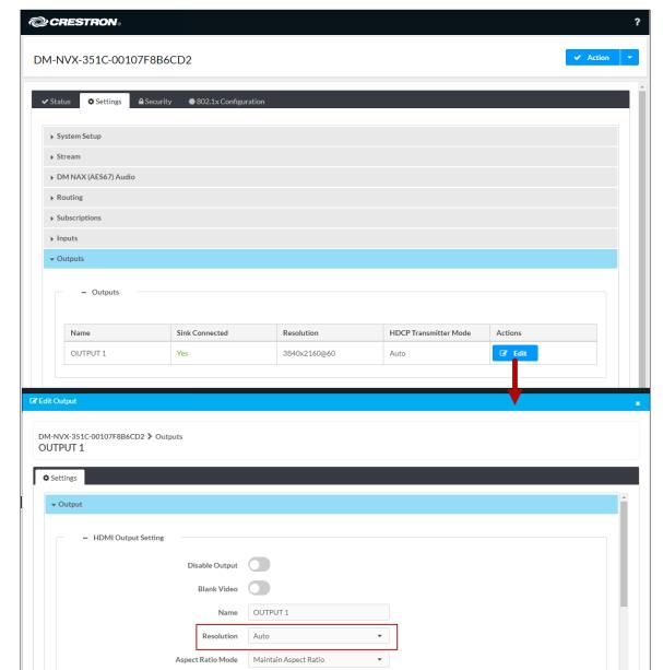
Settings Tab – Outputs, HDMI Output Resolution Configuration
