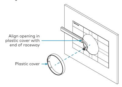
2. While holding the cover in place, tape the outer ring of the cover to the template.
