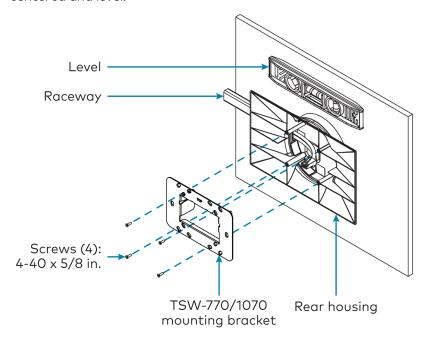
**NOTE:** If installing a TSW-770-LB or TSW-1070-LB light bar as part of the MSMK installation, the light bar must be placed in between the TSW-770/1070 mounting bracket and the MSMK rear housing during this stage of the installation. For more information on installing the light bar, refer to the TSW-770-LB and TSW-1070-LB Quick Start (Doc. 8553).
