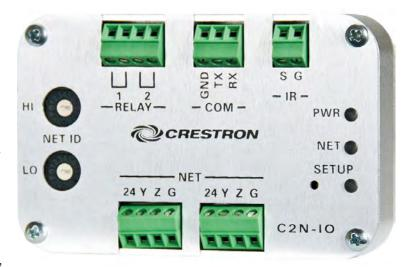
**NET:** (1) amber LED, indicates communication with Cresnet system **SETUP:** (1) red LED and (1) recessed miniature pushbutton for TSID
