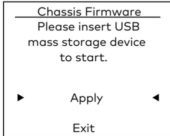
4. Insert a USB flash drive into the USB Type A port, which is located on the front panel of the DMF-CI-8.
