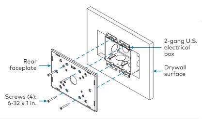
**NOTE:** Four washers are provided to secure the faceplate to the electrical box if the mounting holes are too large for the included screws.
