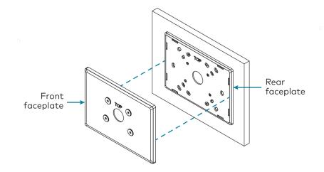
NOTE: If the front faceplate needs to be removed, insert the tip of a flathead screwdriver (or similar tool) into the machined notches on the bottom of the faceplate, and then carefully push against the faceplate to pop it off. Refer to the following image for the location of the notches.
