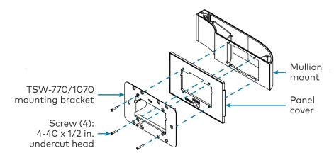
If the TSW-770-LB or TSW-1070-LB light bar will be used in this installation, use the four provided 4-40 x 3/4 in. screws instead of the 4-40 x 1/2 in. screws. The light bar should be placed in between the TSW-770/1070 mounting bracket and the panel cover as shown in the illustration below.
