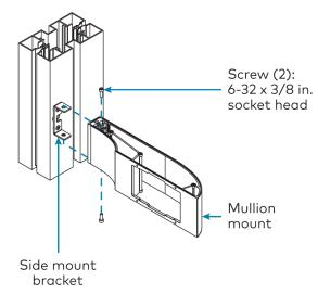
8. Align the TSW-770/TSW-1070 mounting bracket (included with touch screen) with the panel cover as shown in the illustration below, and then secure both to the mullion mount with the four  $4-40 \times 1/2$  in. undercut head screws.
