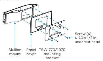
If the TSW-770-LB or TSW-1070-LB light bar will be used in this installation, use the four provided  $4-40 \times 3/4$  in. screws instead of the  $4-40 \times 1/2$  in. screws. The light bar should be placed in between the TSW-770/1070 mounting bracket and the panel cover as shown in the illustration below.
