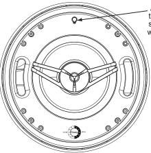
Attach grille safety tether with supplied screw Cover screw with supplied rubber
