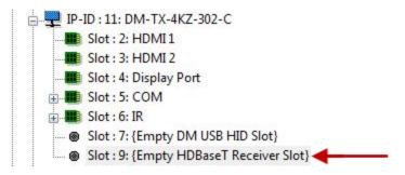
When the third-party HDBaseT receiver device is added to slot 9, the HDBaseT Receiver symbol adds a COM port to the device and enables two-way serial communication.
