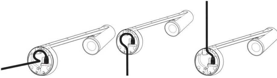
**STEP 3: ATTACH THE CAMERA ONTO THE CAMERA MOUNTING BRACKET**
