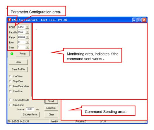
Please set the parameters of COM number, bound rate, data bit, stop bit and the parity bit correctly, and then you are able to send command in command sending area.
