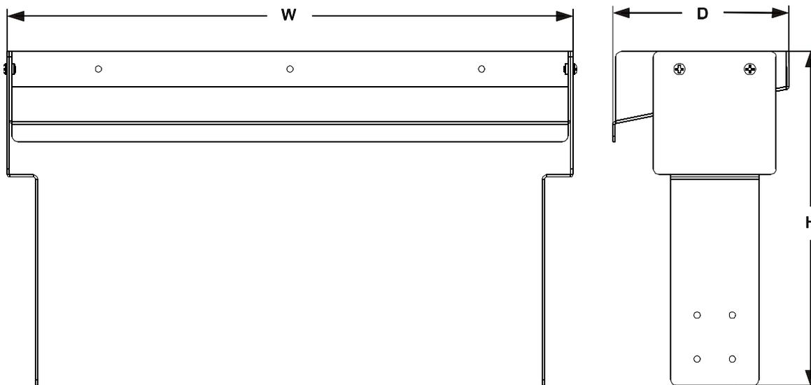
*External Dimensions of CAEN/GLEX-DRS Series Drip Shields*
