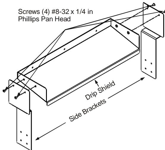
2. Locate the appropriate mounting holes on the lighting enclosure and attach the drip shield using (4) #8-32 x 1/4 inch screws (included) and (4) #8-32 hex nuts (included) as shown below.
