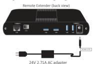
5 Attach USB device(s) to the Remote
