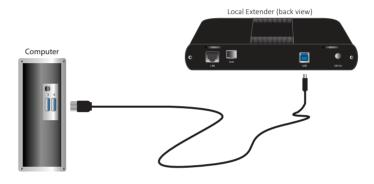
3 Power the Local Extender with the included 24V 1A AC adapter and tighten the locking ring.
