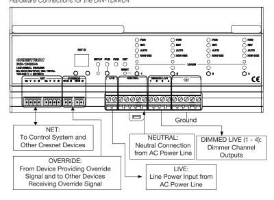
With the circuit breaker turned off, connect the wires to the terminal blocks per the markings provided on the DIN-1DIMU4. When making LIVE, NEUTRAL, DIMMED LIVE, and ground connections, strip the ends of the wires approximately 5/16 in (8 mm). Use care to avoid nicking the conductors. Tighten the connector to 4.5 in-lb (0.5 Nm). The wire gauge should be 10 to 24 AWG.
