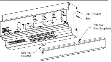
**NOTE**: To remove the DIN-1DIMU4 from the DIN rail, use a small, flat object (i.e., a flat-head screwdriver) to pull the DIN rail release and tilt the bottom of the DIN-1DIMU4 away from the DIN rail.
