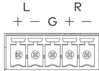
Refer to the following table and diagram for analog audio output pin assignments and connection information.
