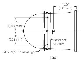
Note: Cabinets are hand-laminated and measurements vary slightly due to the thickness of the fiberglass. Dimensions shown should not be used to fabricate hanging fixtures. Mounting points are approximate.
