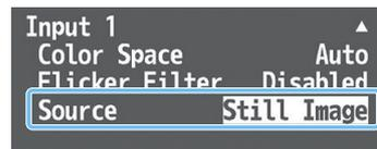
If you select the input channel to which "Still Image" is assigned, the still image is output.
