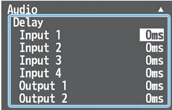
2. Use the VALUE [-] [+] buttons to adjust the delay time of the input audio or output audio.
