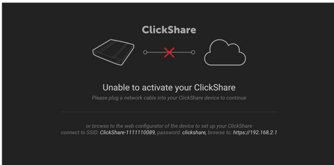
Figure: 'Unable to activate' screen on the Base Unit, shown on first time boot, when no valid network connection can be set up. **Note** that the bottom part of this image, which allows the configuration of a wireless client connection, can only be found on Base Units with production firmware 2.8 or higher.
