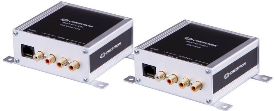
The Crestron<sup>®</sup> AUD-EXT Series is a family of low-cost audio extenders designed for transporting analog and digital audio signals over several hundred feet using inexpensive CAT5 (or better) UTP cable. Three different AUD-EXT models are available, each consisting of one transmitter and one receiver. Models include:
