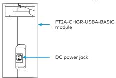
7. Orient the module so that the module's engraved icon is facing toward the front of the FT2 FlipTop assembly.
