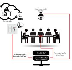
This application diagram highlights the general system connectivity for a networked audio conferencing system utilizing Bluetooth call bridging with Attero Tech's call bridging enabled networked audio products.
