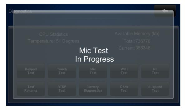
During a microphone test, the built-in microphone records sound for five seconds and then plays the sound back to confirm it is functioning. When the playback is finished, the display automatically returns to the **Diagnostics** screen.
