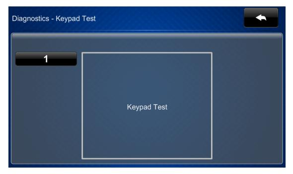
Use the **Diagnostics - Keypad Test** screen to test the functionality of the reset button on the rear of the touch screen. When the reset button is pressed, its respective indicator lights on the screen.
