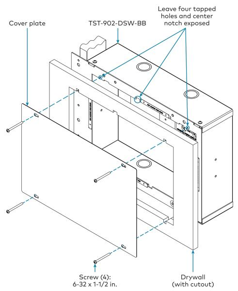
Remove the cover plate and 6-32 x 1-1/2 in. screws (if used), and then install the TST-902-DSW wall dock into the TST-902-DSW-BB as described in Install the TST-902-DSW on page 47 with the 6-32 x 1-1/2 in. screws.
