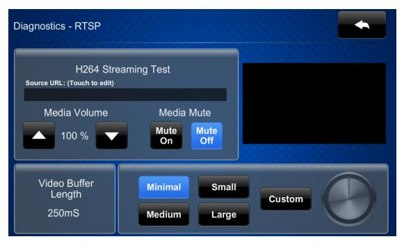
Use the **Diagnostics - RTSP** screen to view and test RTSP (real time streaming protocol) on the touch screen.
