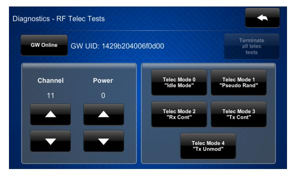
The **Diagnostics - RF Telec Tests** screen provides controls that can be used to perform various Telec tests, including changing the RF channel and power level.
