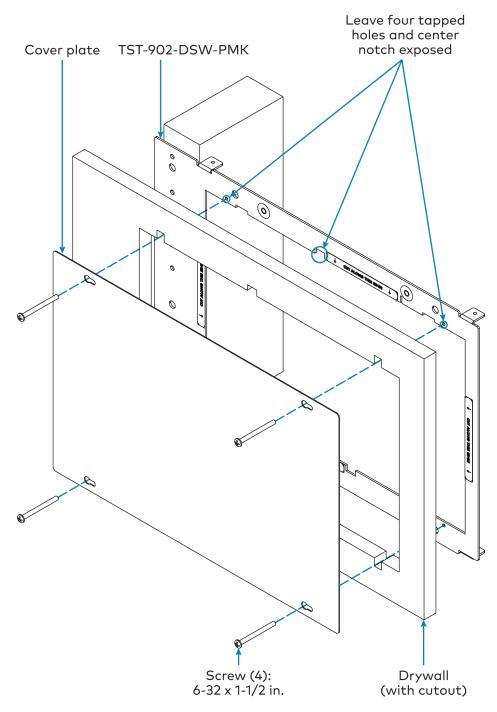
8. Remove the cover plate and 6-32 x 1-1/2 in. screws (if used), and then install the TST-902-DSW wall dock into the mounting bracket as described in Install the TST-902-DSW on page 47 with the 6-32 x 1-1/2 in. screws.
