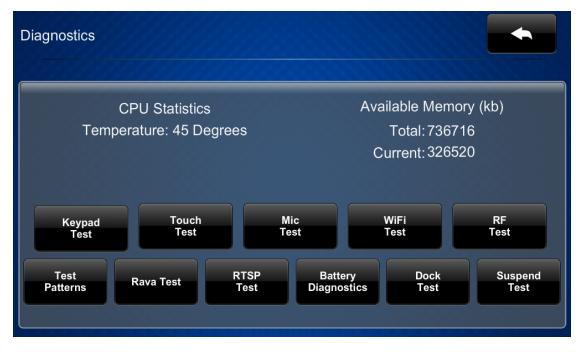
Use the **Diagnostics** screen to access various diagnostic test screens for the touch screen. The **Diagnostics** screen also provides the touch screen CPU temperature and available memory.
