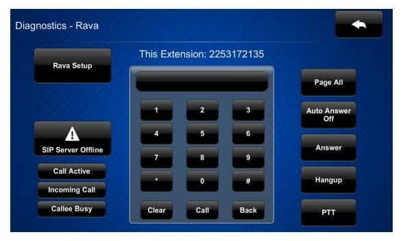
Use the **Diagnostics - Rava** screen to test using the Rava® SIP Intercom with the touch screen. Rava SIP intercom technology enables hands-free VoIP communication with other Rava-enabled touch screens and door stations. Rava works over Ethernet, supporting 2-way intercom and paging without requiring any special wiring.
