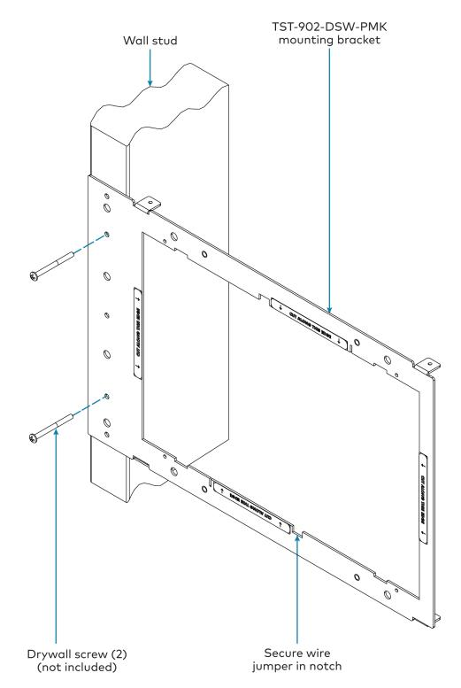
5. Route any wiring for the TST-902-DSW through the opening in the mounting bracket and secure them into the wire jumper.
