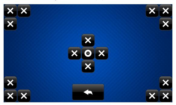
Use the touch test screen to test the touch functionality of the display. When a location button is tapped, its respective indicator lights on the screen.
