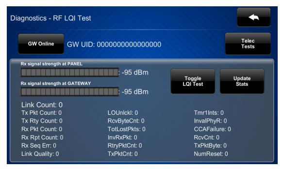
Use the **Diagnostics - RF LQI Test** screen to view and test the RF connection to an Extended Range gateway. Statistics for the RF connection are displayed, as well as controls to toggle the RF LQI (link quality indicator) test and to update the connection statistics.
