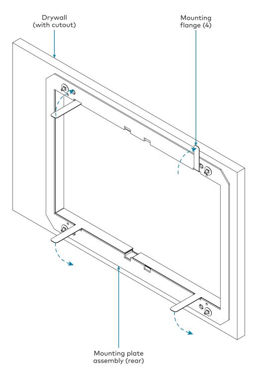
9. Use four standard drywall screws to loosely secure the mud ring to the mounting plate and adjustment plate assembly. The screws must pass through the clearance holes in the mounting plate to be secured in the extruded holes of the adjustment plate.
