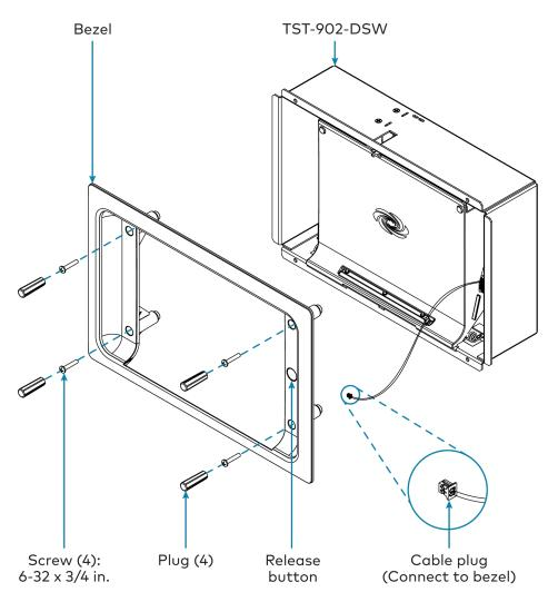
8. Test the installation by pushing the release button on the right of the bezel to open the cradle. Then, push the cradle back into place to close it.
