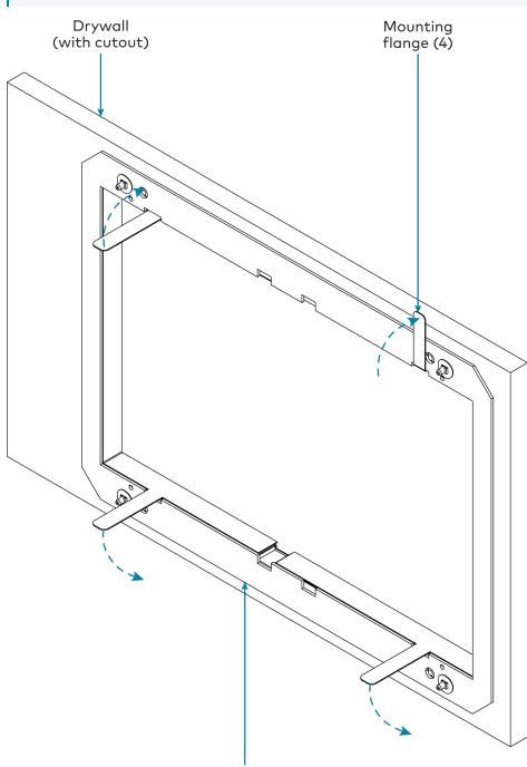
**NOTE:** The mounting plate has a slight amount of play. This is normal, as it allows for minor adjustments to be made to the TST-902-DSW during installation.
