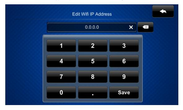
The on-screen numeric keypad opens for the chosen setting.
