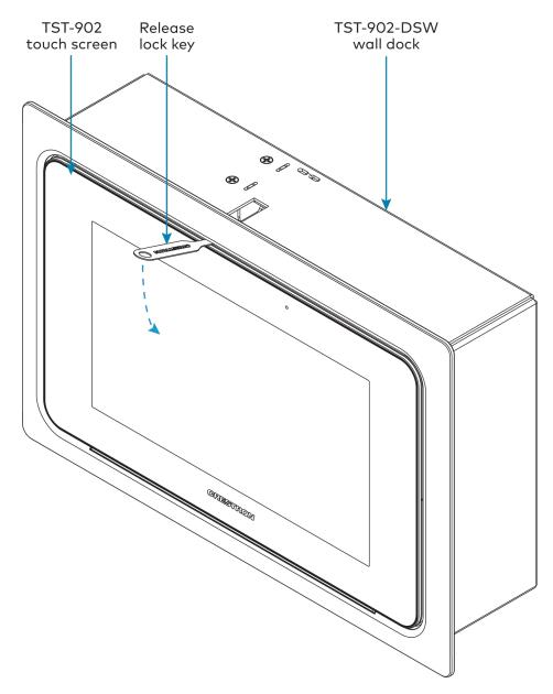
3. Remove the key to open the cradle so that the touch screen can be removed.
