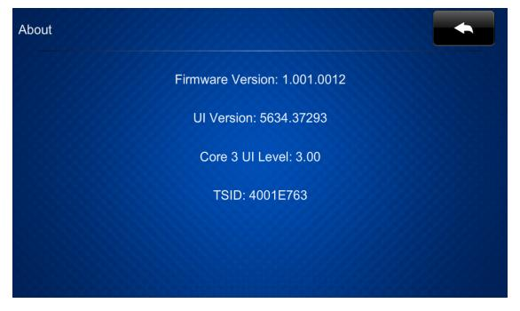
Use the **About** screen to view information about the touch screen, including the firmware version and the operating system versions.
