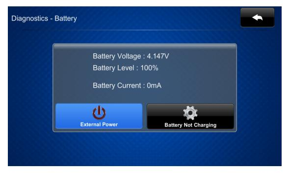
Use the **Diagnostics - Battery** screen to view the TST-902 battery voltage, charge, and current levels.
