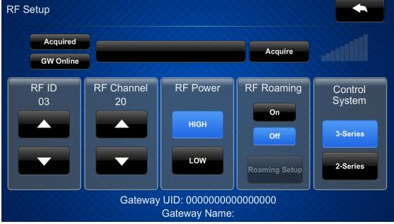
The **RF Setup** screen provides controls that can be used to acquire the TST-902 to a Crestron Extended Range (ER) wireless gateway (not included). Once the TST-902 has been acquired to a gateway, the gateway UID, name, and RF signal strength are displayed.
