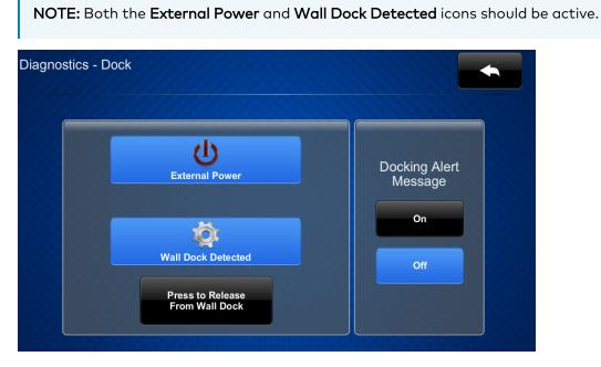
3. Tap **Press to Release From Wall Dock**. The cradle will open automatically so that the touch screen can be removed.
