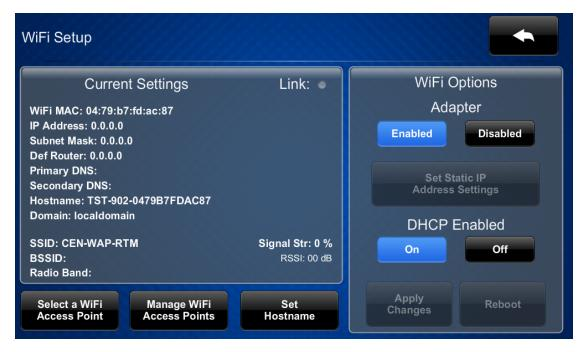
Use the **Wi-Fi Setup** screen to view the Wi-Fi network MAC and IP addresses, subnet mask address, default router address, primary and secondary DNS addresses, host name, domain, and various details about the Wi-Fi connection. A **Link** indicator is provided to indicate the status of the Wi-Fi connection. (Green indicates that the Wi-Fi connection is active.)
