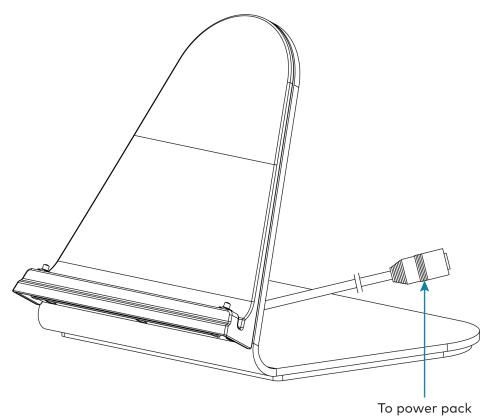
After power has been applied to the TST-902-DS, place the TST-902 touch screen on the TST-902-DS by aligning its three charging contacts with the bottom of the charging dock. The touch screen should be seated firmly on the charging dock once attached, and the touch screen battery will begin to charge.
