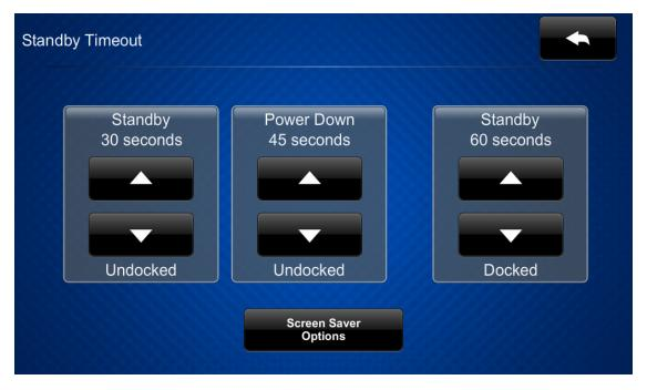
Use the **Standby Timeout** screen to set the standby timeout settings for the touch screen.
