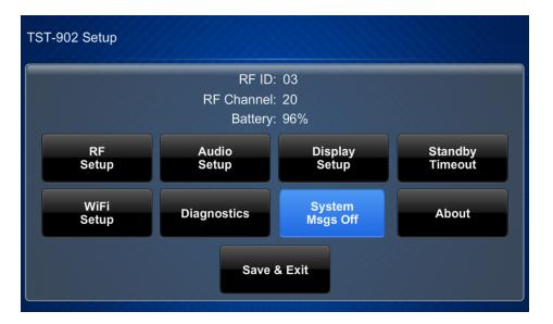
2. Tap Wi-Fi Setup. The Wi-Fi Setup screen is displayed.
