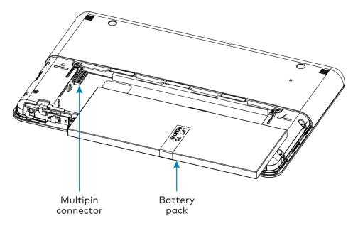
6. Ensure the pin side of the multipin connector on the TST-902 is facing upward, and then connect it to the battery pack wire harness as shown in the following image.
