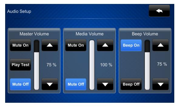
Use the **Audio Setup** screen to control the main volume, media volume, and beep volume settings for the touch screen.
