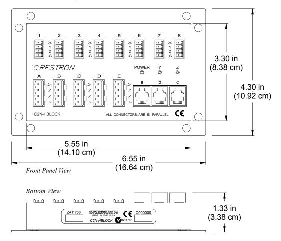
There are three LEDs on the front panel of the C2N-HBLOCK. The LED labeled **POWER** illuminates when 24VDC is attached to one connector and is available at the remaining connectors. The **Y** and **Z** data signal LEDs are used to diagnose wiring problems of the data signal input to the C2N-HBLOCK. Refer to "Y and Z LED Illumination" on page 9 for further information.
